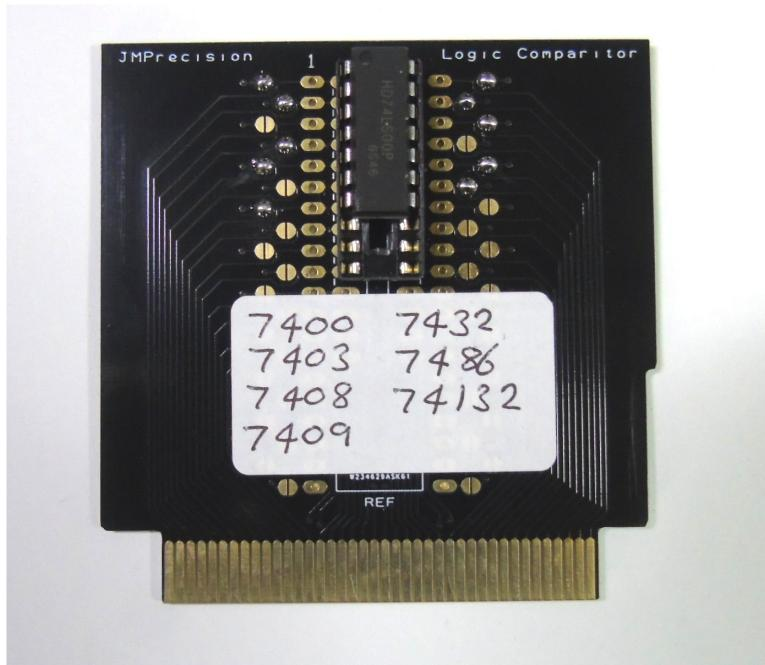
This module is configured for testing 74LS00 devices. Note the shorted jumpers for all the inputs and power pins. The label shows other devices with the same pin configuration which can also be used with this same module configuration.
